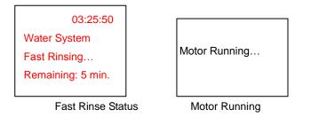
•The working process is Service $\rightarrow$  Backwash $\rightarrow$  Brine& Slow Rinse $\rightarrow$  Brine Refill  $\rightarrow$ Fast Rinse $\rightarrow$  Service (Cycle repeats).
