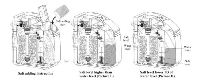
%Please strictly use the salt of more than 99% purity only. Any salt with additive or large particles is forbidden to add.
